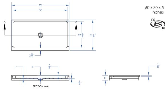
FEATURES Dimensional Tolerance ± %", Dimensions needed for site preparation should be measured from the unit. Dadi assumes no responsibility for preparatory work.
